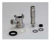
8. The under the bar piston have to be disassembled before push out of the body. Therefore unscrew lower and upper part and remove it from the housing.
