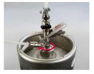
15. Reconnect the dispense head to the beverage container. Push the dispense heads A-type and combi onto the disc of the spear respectively turn the dispense heads S-type, G-type and Draft into the spear clockwise.
