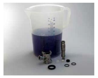
9. Lay the single components of the dispense head in a cleaning agent and disinfectant and allow it to react (reaction time prescribed by the agent).
