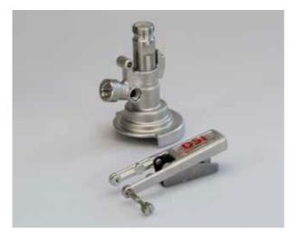
6. Remove the knurled screw in order to remove the grip. Pull the grip components from the body and the piston.
